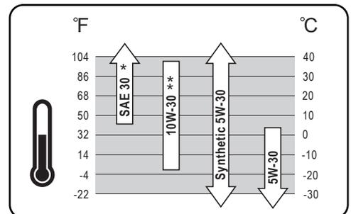
Note: \*Below 40°F (4°C) the use of SAE 30 will result in hard starting. \*\*Above 80°F (27°C) the use of 10W-30 may cause increased oil consumption. Check oil level more frequently
