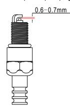
Standard Spark Plug: E6TC/E6RTC/BPR6HS
