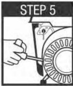
Pull the starter grip lightly until you feel resistance, then pull briskly to start the engine.
