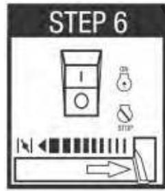
Move the choke lever to the "OPEN" position.
